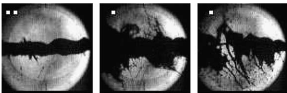
Fig. 4. Photographs of a 1 cm mercury jet struck by a pulse of 2 \times 10^{12} 24 GeV protons [5].
